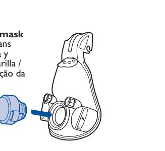
Assembled valve inserted into mask
